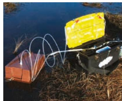
*Floating chamber measuring greenhouse gas fluxes from a pool surface*
