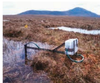
*Logging equipment recording water level and temperature*
