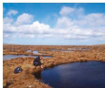
*Sampling for analysis of dissolved carbon dioxide in the pool water*
